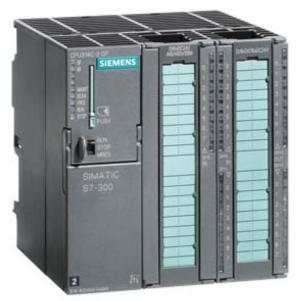
SIMATIC S7-300, CPU 314C-2 DP COMPACT CPU WITH MPI, 24 DI/16 DO, 4AI, 2AO, 1 PT100, 4 FAST COUNTERS (60 KHZ), INTEGRATED DP INTERFACE, INTEGRATED 24V DC POWER SUPPLY, 192 KBYTE WORKING MEMORY, FRONT CONNECTOR (2 X 40PIN) AND MICRO MEMORY CARD REQUIRED
