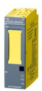
SIMATIC DP, ELECTRON. MODULE FOR ET200SP, F-RQ 1X24VDC/24..230VAC/5A ST, 20MM WIDTH, 1 RELAY OUTPUT (2 NO-CONTACTS) TOTAL OUTPUT CURRENT 5A, RATED VOLTAGE DC 24V AND AC 24 .. 230V, USEABLE UP TO PL E (ISO13849-1: 2008)/ SIL 3 (IEC61508: 2010) IF CONTROLLED BY A F-DQ (E.G. 6ES7136-6DB00-0CA0)
