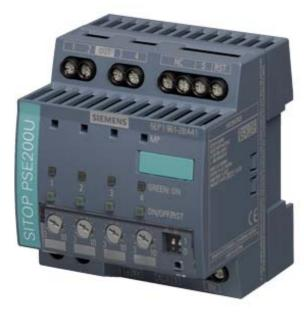
SITOP PSE200U SELECTIVITY MODULE 10A SITOP PSE200U 10 A Selectivity module 4-channel input: 24 V DC/40 A output: 24 V DC/4x 10 A Level adjustable 3-10 A mit status message for each output
