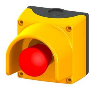
ENCLOSURE FOR COMMAND DEVICES, 22MM, ROUND, ENCLOSURE MATERIAL PLASTIC, YELLOW ENCLOSURE TOP PART, WITH PROTECTIVE COLLAR, 1 COMMAND POINT, A=EM. STOP MUSHROOM PUSHB. RED, 40MM, ROTATE-TO-UNLATCH, 1NC, SCREW TERMINAL, FLOOR MOUNTING, TOP AND BOTTOM 1 X M20 EACH !!! Phased-out product !!! SIRIUS ACT 3SU1 is successor Preferred successor type is >>3SU1801-0NA00-2AC2<<
