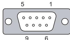
Pin assignment of the RS 422/RS 485 interface
