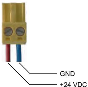
Connect the plug-in terminal strip to the cables of the power supply as shown in the figure above. Ensure that the lines are connected properly to the correct terminals. Refer to the label for the contact pins on the rear of the HMI device.
