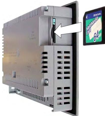
When inserting the memory card, please note that it can only be inserted as shown in the diagram. The memory card is inserted correctly in the memory card slot when the card lock engages.
