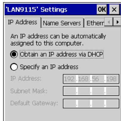
2. If you need automatic issuing of addresses, select the "Obtain an IP address via DHCP" radio button.
