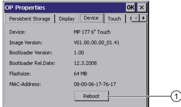
① Button for restarting the HMI device
