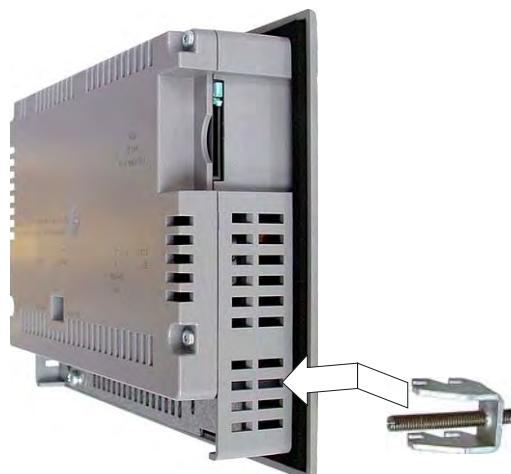
4. Fasten the mounting clamp by ① tightening the set screw ②.
