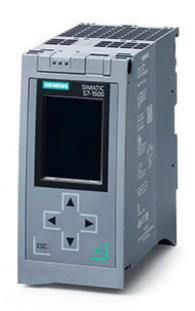
SIMATIC S7-1500F, CPU 1515F-2 PN, CENTRAL PROCESSING UNIT WITH WORKING MEMORY 750 KB FOR PROGRAM AND 3 MB FOR DATA, 1. INTERFACE: PROFINET IRT WITH 2 PORT SWITCH, 2. INTERFACE: PROFINET RT, 30 NS BIT-PERFORMANCE, SIMATIC MEMORY CARD NECESSARY
