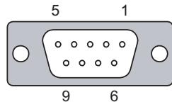
Pin assignment of the RS 422/RS 485 interface
