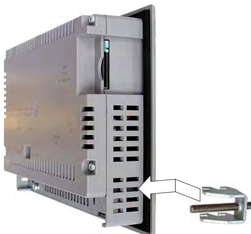
4. Fasten the mounting clamp by ① tightening the set screw ②.
