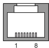
Pin assignment of the RJ45 connector
