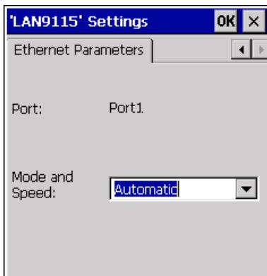
"Automatic" is preset in the field "Mode and Speed" for the data rate and transmission rate of the Ethernet connection. With this setting, the HMI device automatically detects the data rate and speed of communication via Ethernet and adapts to this.
