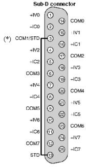
+IVx + pole voltage input for channel x
