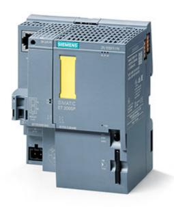
SIMATIC DP, CPU 1510SP F-1 PN for ET 200SP, Central processing unit with Work memory 150 KB for program and 750 KB for data, 1st interface: PROFINET IRT with 3-port switch, 72 ns bit performance, SIMATIC Memory Card required, BusAdapter required for Port 1 and 2
